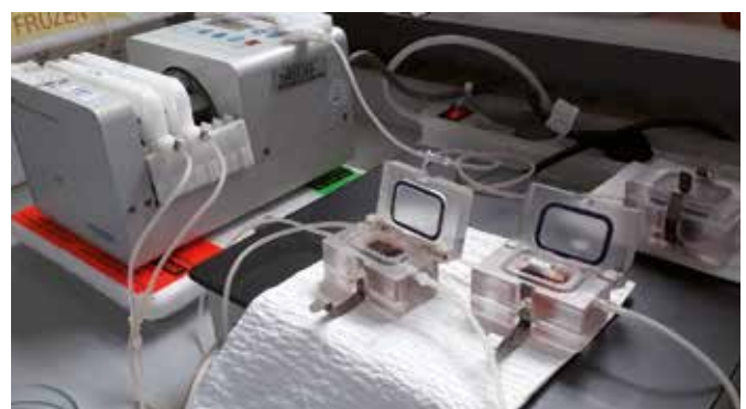
Figure 2: RPE/choroid rings in perfusion chambers. Media samples of a fucoidan treated and an untreated organ culture are taken after passing through the chamber, to compare the VEGF secretion.
